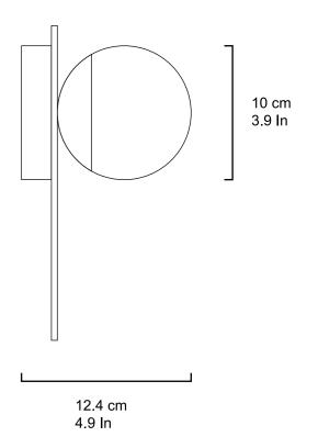
240V / 110V Illumination: Socket: G9 Bulb: 1 x 5 Watt G9 LED Wattage: 5W Lumens: 420 Temprature: 2700K Color: Warm White Bulb Life: 30,000 Hours Dimmable
